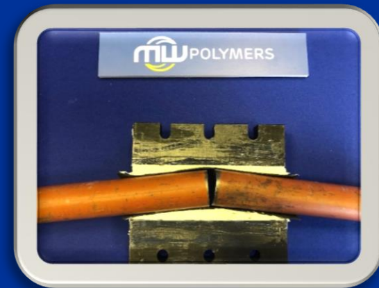
Image shows a cut-away through the rubber sleeve with cured resin
