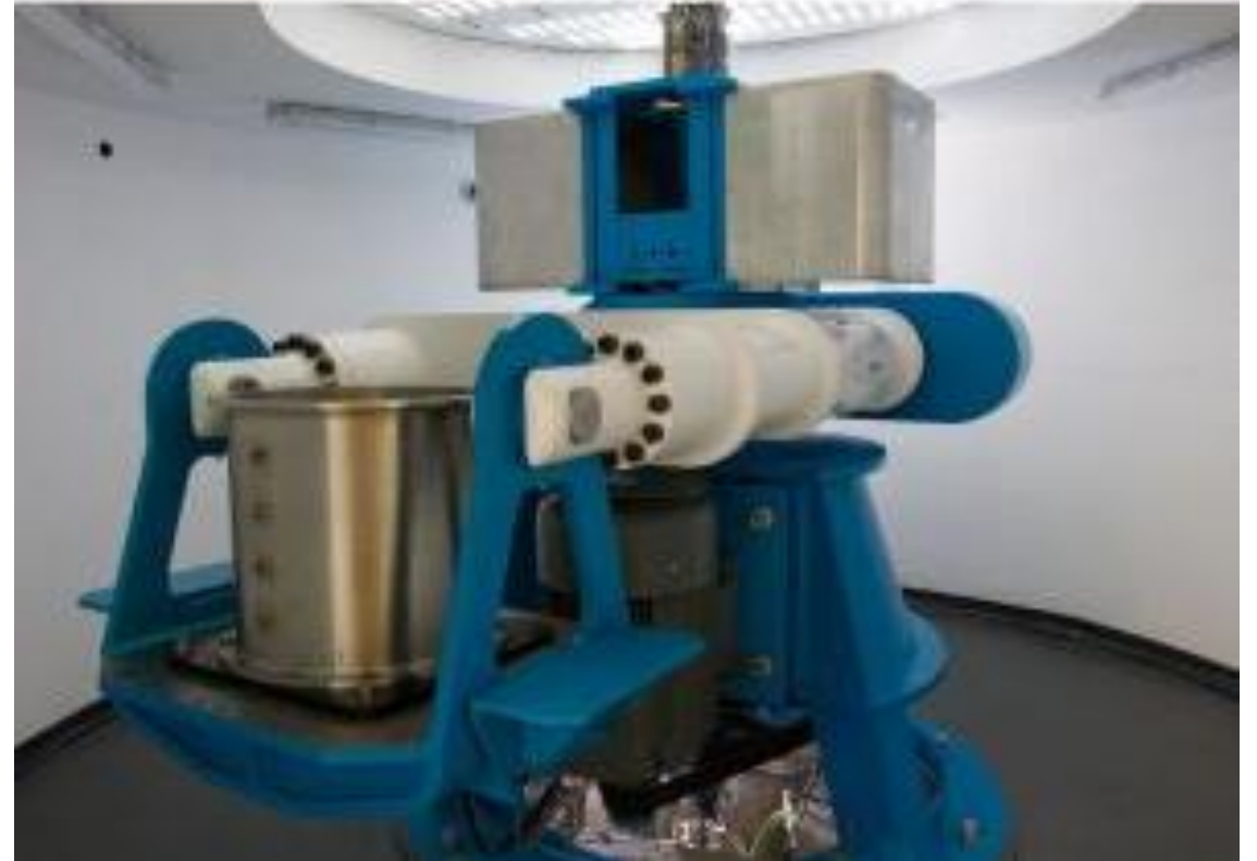
University of Sheffield's 50-gT 4m diameter geotechnical beam centrifuge
